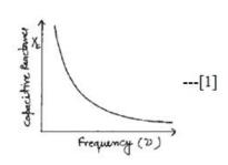
(d) (i) For ac  $X_c$  is finite and therefore allows the ac to pass. --[1/2]
