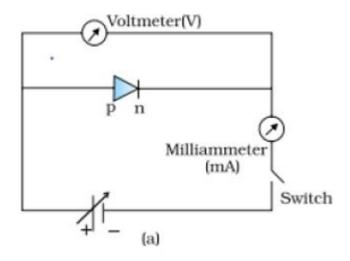
[b] features of t (i) forward biasing, and (ii) reverse biasing [1/2 + 1/2]
